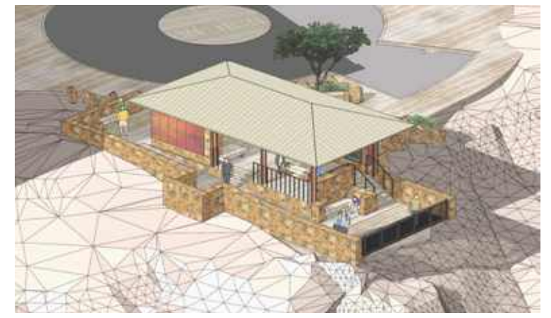
The site contours provided by the Landscape Architect allowed me to make a realistic 3D topo model (CAD & Sketchup)
